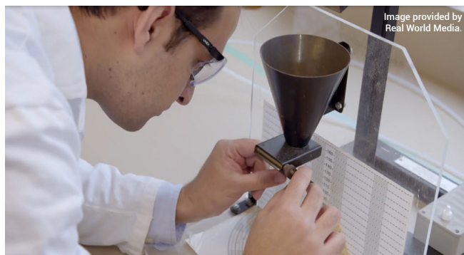
Dr. Hamid Rezaei is measuring the angle of repose of wheat straw.
