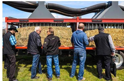
Figure 3. A new hay dryer (Ag Maximizer) design and built in Prince George BC and demonstrated at AgSmart. The heated air enters the baled hay through a series of vertical tubes penetrated into the large square bale. The sources of heated air is the heat recovery from a 375 hp diesel engine that runs the high pressure blower
