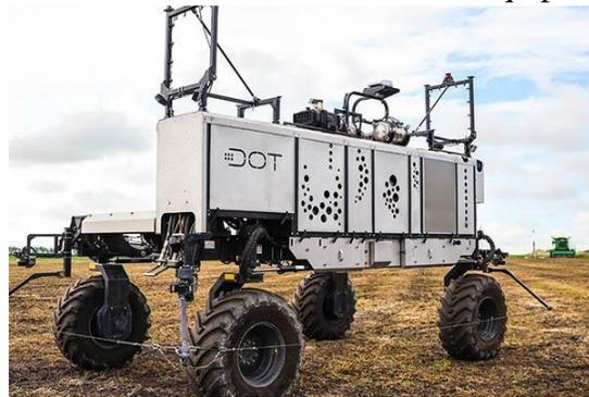
Figure 2. DOT driverless (autonomous) sprayer demonstrated at the Ag-Smart event
